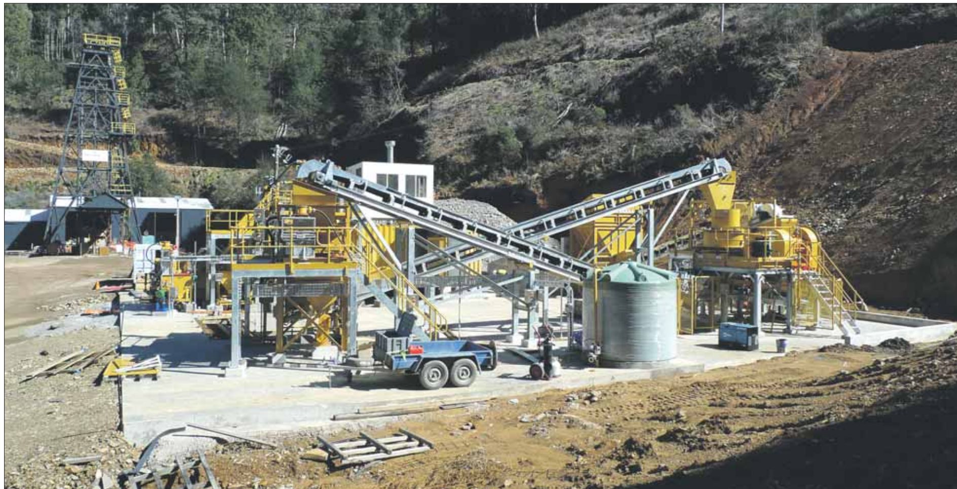
High hopes: Morning Star Gold's onsite gravity processing plant (GPP) is designed to process ore at the rate of 10 tonnes per hour.
